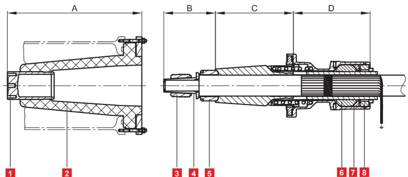
Sample Drawing: Cable connecting system CONNEX Size 5
